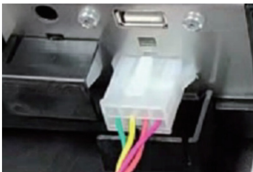
9. Connect cable to the coffee machine.
