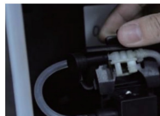
4. Open front panel, press as the buckle and pull up the nozzle of milk frother.
