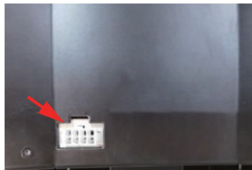
10. Connect cable to the syrup station.
