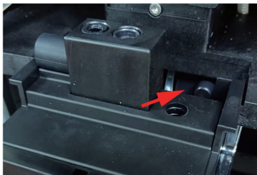
8. Insert syrup tubes into dispensing position and connect the milk frother again.
